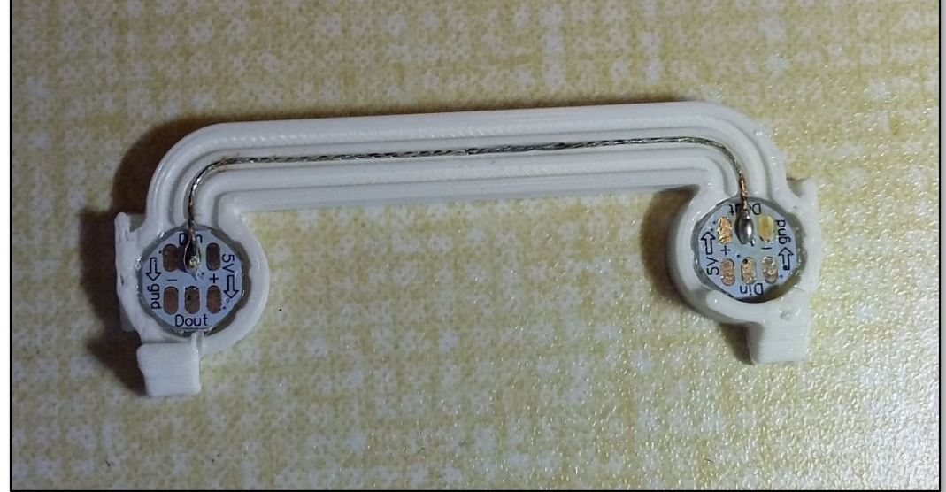
02 RGB LEDs glued into position and data wire attached
