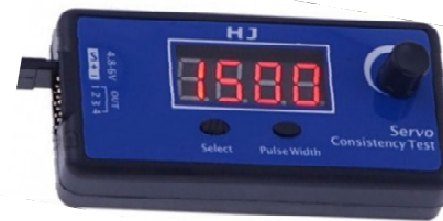
HJ servo tester displays pulse widths directly in µs.
